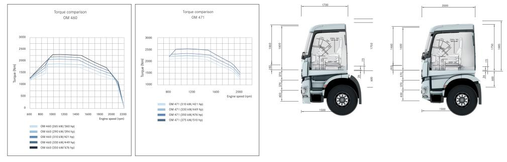
More power - less fuel. From 265 kW /360 hp to 350 kW/476 hp (OM 460) and from 310 kW/ 421 hp to 375 kW/ 510 hp (OM 471), these engines make their maximum torque available in the lower, fuel-efficient engine speed range. Engine tunnel: 170 mm Standing headroom on engine tunnel: 1460 mm
