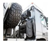
Air filter system. Dust and sand in the intake air is a serious problem for the engine. That is why Mercedes-Benz firstly uses a cyclone pre-filter that already removes as much as 80% of the dust. Secondly, the filter papers used are much larger than those normally used in Europe, to trap the remaining 20% effectively. A neat solution for engines that are already having to work hard.
