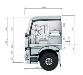
Engine tunnel: 170 mm Headroom on engine tunnel: 1460 mm Headroom in front of the seats: 1590 mm
