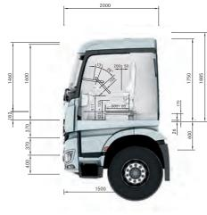
Engine tunnel: 170 mm Headroom on engine tunnel: 1460 mm Headroom in front of the seats: 1600 mm
