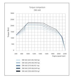
More power – less fuel. From 265 kW (360 hp) to 350 kW (476 hp) the OM 460 engines make their maximum torque available in the lower, fuel-efficient engine speed range.
